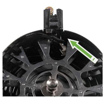
Load 3 rounds of 7.62x39mm ammunition (pointed down) into the outermost feed track in front of the follower and rotate the feed wheel counterclockwise too feed the first 3 rounds into the feed tower.
