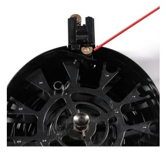
Load one round into the remaining space of the feed ramp just below the feed tower.
