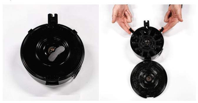
Place the drum face down on a flat surface with the feed tower at the 12 O'clock position and unlatch the two hinged lid latches by lifting them up and towards the feed tower. Open the loading lid.
