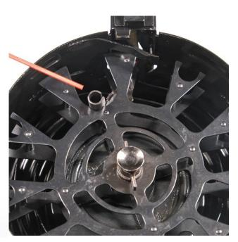
Depress and hold the spring tension release button and rotate the feed wheel clockwise until the follower stops around the 11 O'clock position in the inner most feed track.
