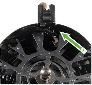
Load 3 rounds of 7.62x39mm ammunition (pointed down) into the outermost feed track in front of the follower and rotate the feed wheel counterclockwise to feed the first 3 rounds into the feed tower.
