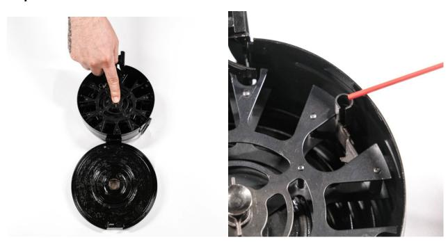
Depress the spring tension release button at the center of the drum and release all spring tension. The amount of pressure needed will depend on how much tension is on the spring. It may be difficult. Rotate the feed wheel and place the follower at the two O'clock position making sure the follower is in the outermost feed track.
