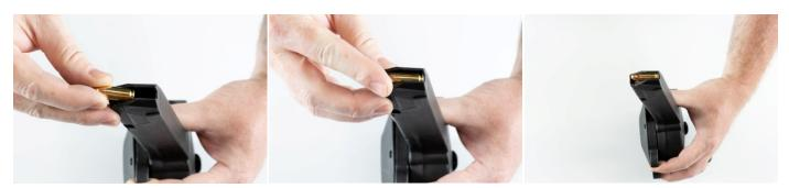
Note: As the drum magazine becomes full, a cartridge may stick in the feed lips from the spring pressure. You may need to gently press on it or lightly tap the drum magazine on a hard surface to dislodge it. At 35-40 rounds you will notice a decrease in spring pressure. This is normal. The rounds are coming up and over the top of the internal spiral feeding track.
