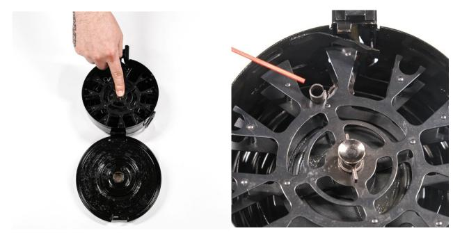
Depress and hold the spring tension release button and rotate the feed wheel clockwise until the follower stops around the 11 O'clock position in the inner most feed track.
