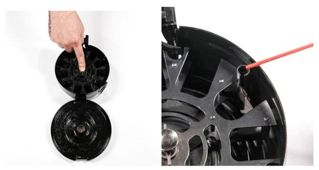
Depress the spring tension release button at the center of the drum and release all spring tension. The amount of pressure needed will depend on how much tension is on the spring. It may be difficult. Rotate the feed wheel and place the follower at the two O'clock position making sure the follower is in the outermost feed track.
