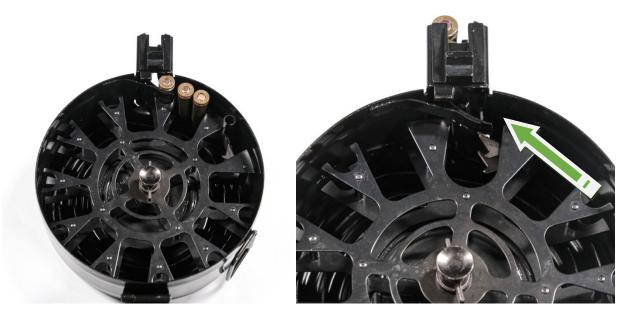
Load 3 rounds of 7.62x39mm ammunition (pointed down) into the outermost feed track in front of the follower and rotate the feed wheel counterclockwise to feed the first 3 rounds into the feed tower.
