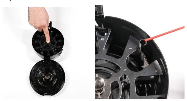
Depress the spring tension release button at the center of the drum to release all spring tension. If needed, rotate the feed wheel and place the follower at the 2 O'clock position making sure the follower is in the outermost feed track.
