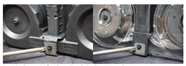
Reposition the magazine floorplate and install using the two screws shown.
