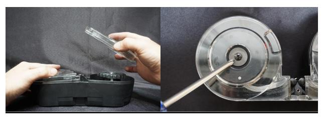
To reassemble, start by replacing the two rear covers and reinstalling the two screws that hold the covers to the drum.
