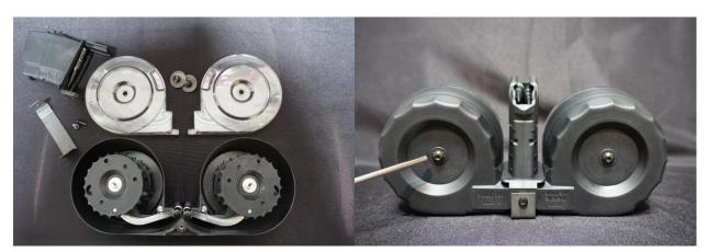
No further disassembly is required beyond the point shown here. Any maintenance or clearing of a malfunction can be done without further disassembly. **WARNING**: At no point should you remove the two screws on the front side of the drum. These screws retain the spring mechanism. Removal of these screws will cause the spring mechanism to dismantle and cannot be reassembled by the user.
