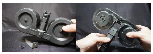
Set the floorplate and screws to the side and separate the tower from the magazine body. **NOTE** - Holding the magazine upside down will help to contain the followers inside the tower during disassembly.
