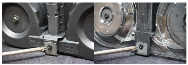
To begin disassembly, start by removing the two screws holding the floorplate to the magazine tower.
