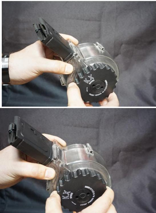
To begin loading, rotate the load assist counter clockwise and insert cartridges, one at a time, into the magazine tower. Using your thumb to brace against the right side of the drum body as shown will provide leverage when rotating the assist.
