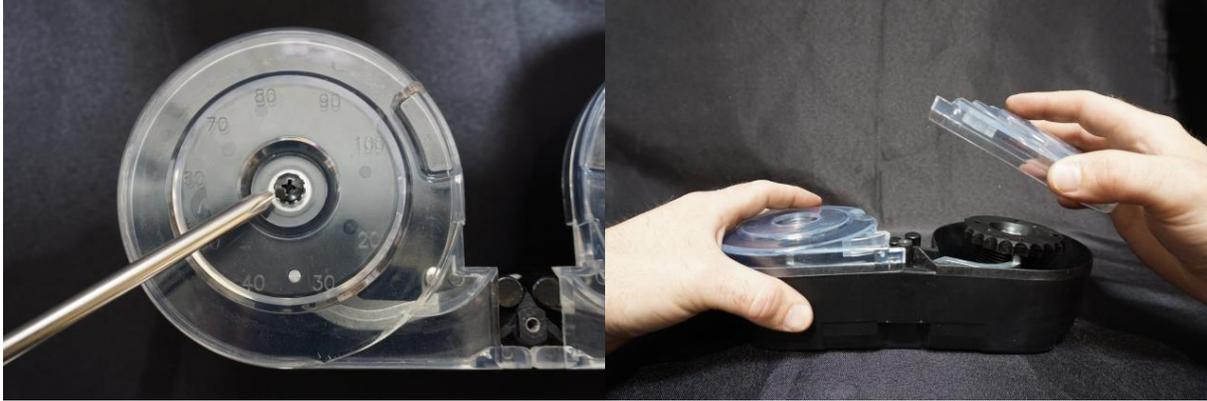
Remove the two screws in the center of the clear covers and set aside. The rear covers will then separate from the body by prying the covers up and outward from the center of the magazine body. This separation may require considerable force. Prying with tools is **NOT RECOMMENDED** as damage to the covers may occur.
